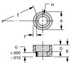
Alternative to lockscrews when using the "fixed" side of a slip-fixed SF bushing. Round clamps have less clearance under their heads, to clamp bushings tighter (which is why you cannot use them on the bushing's "slip" side). Use them with a Socket-Head Cap Screw.
